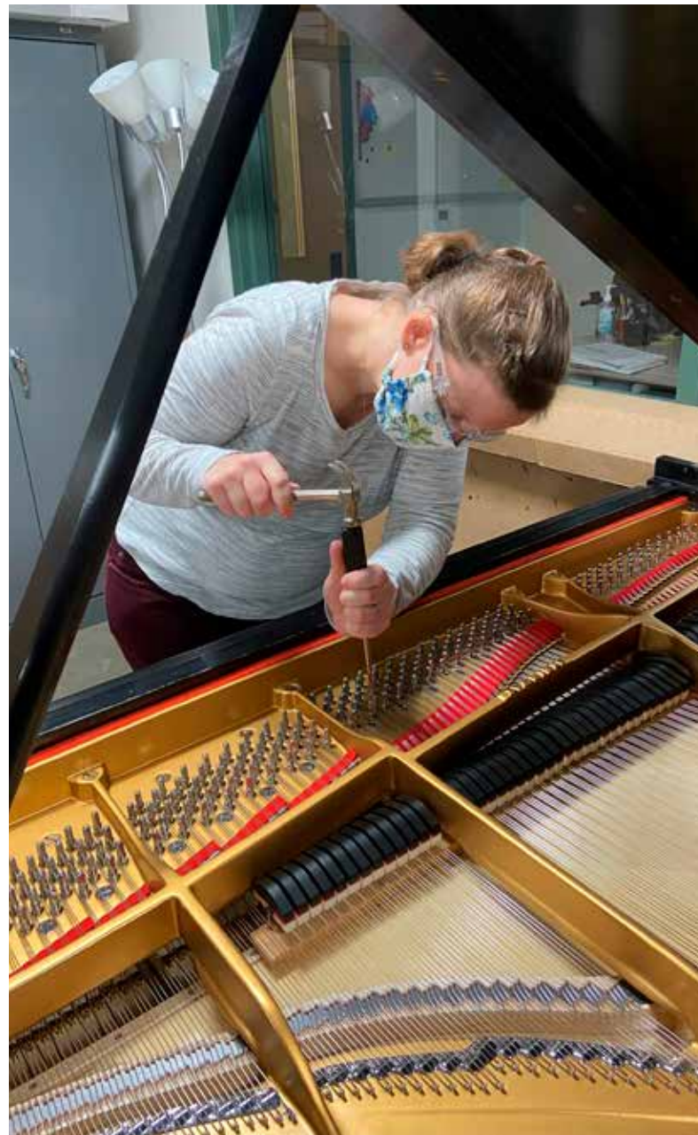
Mary Lapprand studied piano for 10 years and has been the college’s head piano technician for the past five years. Here, she works in the main part of the Carr Piano Shop, tightening string coils on tuning pins on a recently restrung piano.
